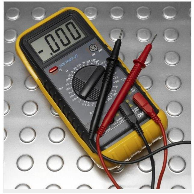
A multimeter can locate ground faults in fire alarm circuits.
